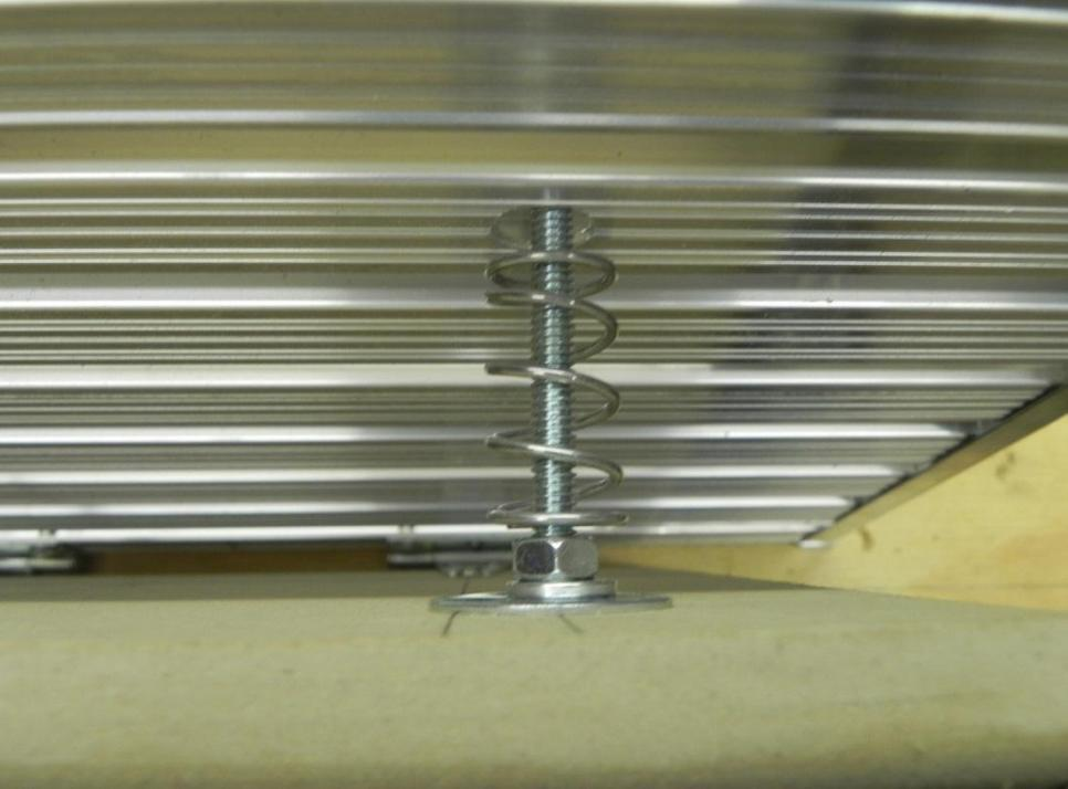
Add springs to the carriage bolts and pass through the holes in the bench. Secure on the backside using fender washer and nylon locknut. The washers will 'bang' on the backside of the bench so I glued foam washers to the fender washers. Felt, foam or other cushioning material can also be used.
