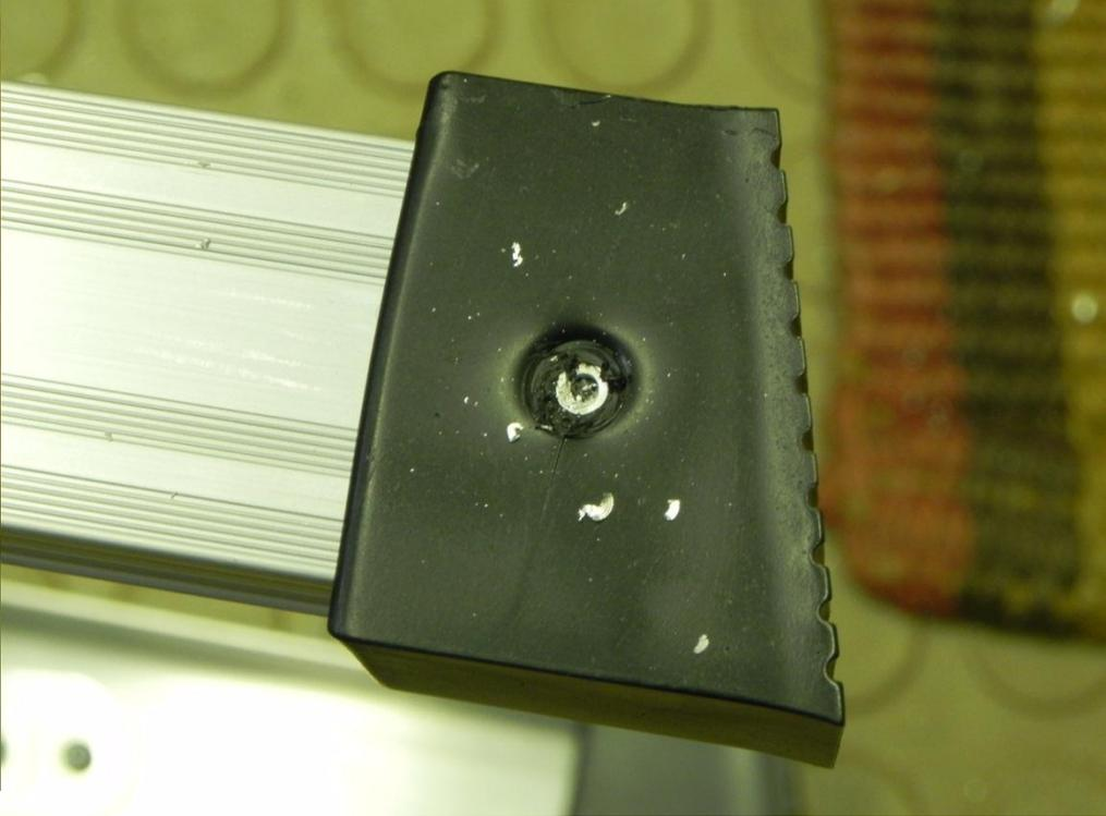
The rubber feet need to be removed. Drill out the head of the rivet and remove foot. You may need to pry a little around rivet.
