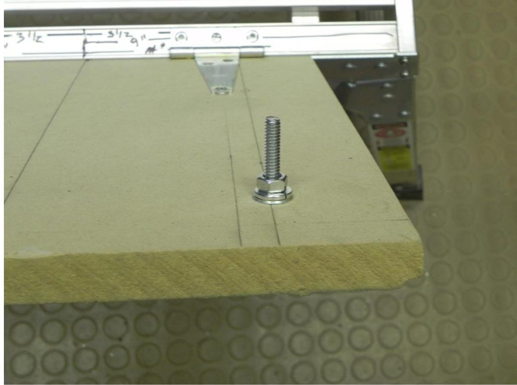
Attach carriage bolt to seat using flat washer and lock washer
