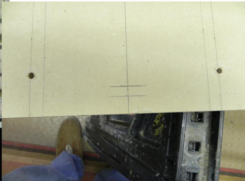
The switch will be activated with a dowel mounted in the seat passing through this space. Using the bench as a guide mark both sides of the gap on the centerline of the seat.
