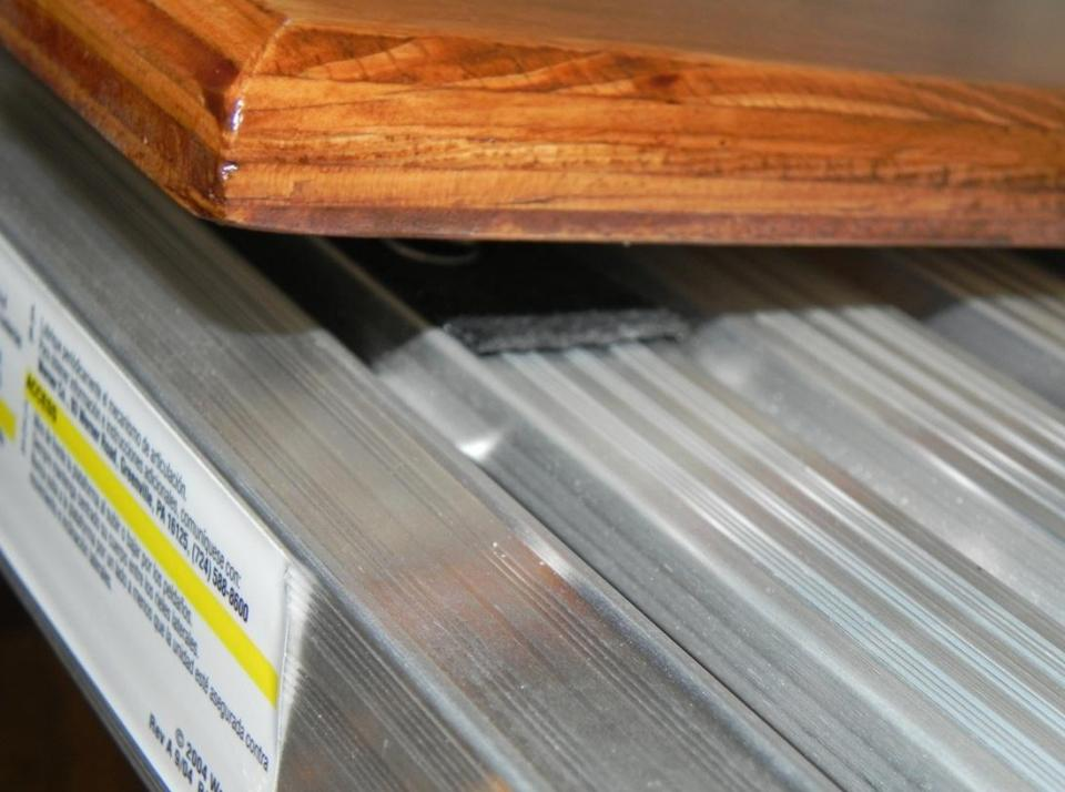
I used some peel and stick felt where the legs support the platforms. These benches tend to be a little 'creaky' and I am hoping the felt quiets them down. The first experience was positive. We'll see how it holds up over time. I also used the felt on the washers and where the springs touch the platform.
