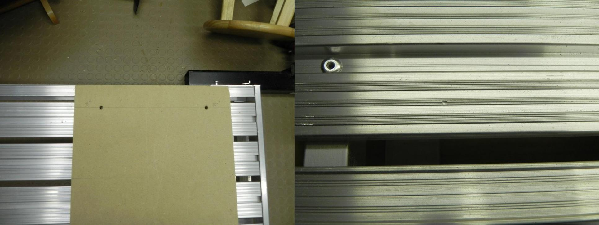
With seat attached to the bench use the 2 holes drilled in the seat to mark hole locations on the bench
