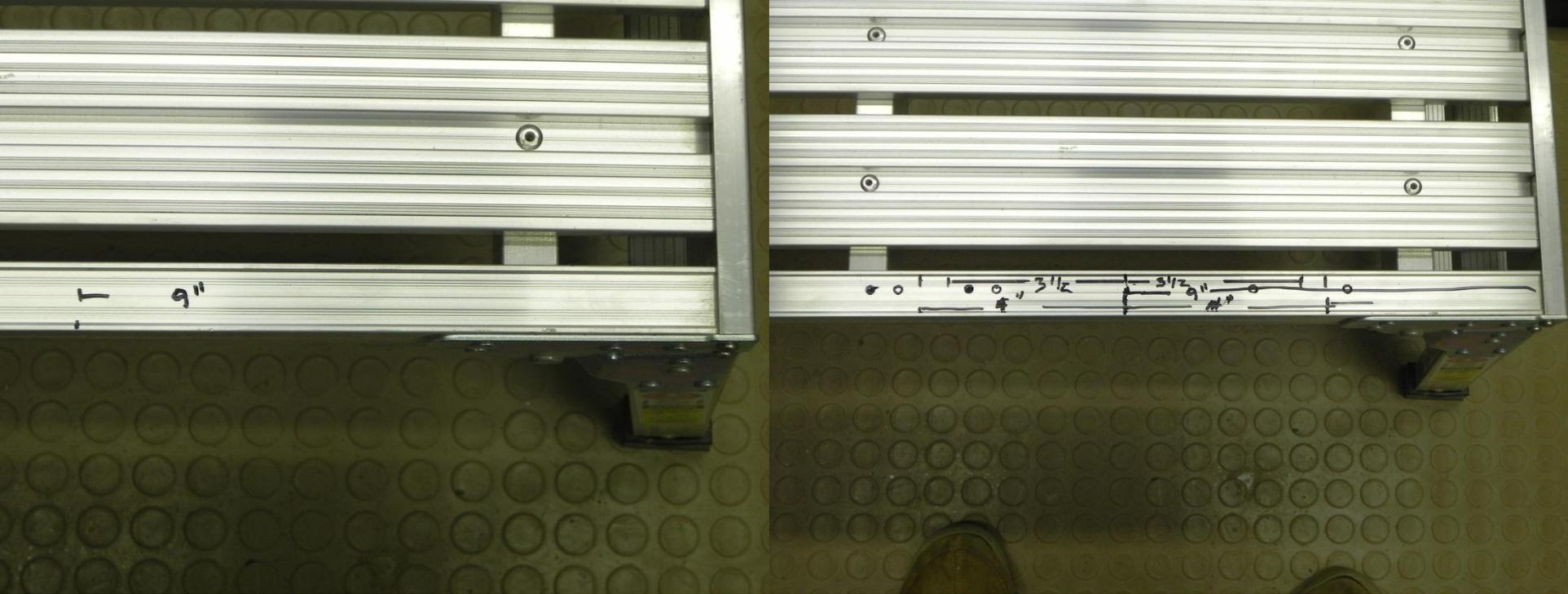
Mark centerline of seat 9" from edge of bench. Use seat with hinges attached. Align centerlines and mark mounting locations for hinges on bench. Drill holes in bench and attach hinges. (I used rivets to attach hinges. It was easier to remove hinges from seat, rivet them to the bench and then reattach the seats.
