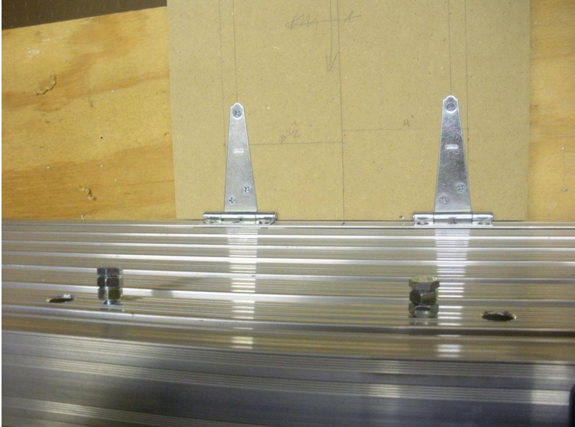
I used bolts with spacers (2 nuts) as rests for the seat. This supports the seat and prevents the switch from being over traveled.
