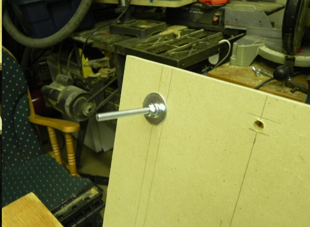
Drill a hole  $\frac{1}{2}$ " deep taking care not to drill all the way through. A dowel will be glued in this hole later to activate switch.
