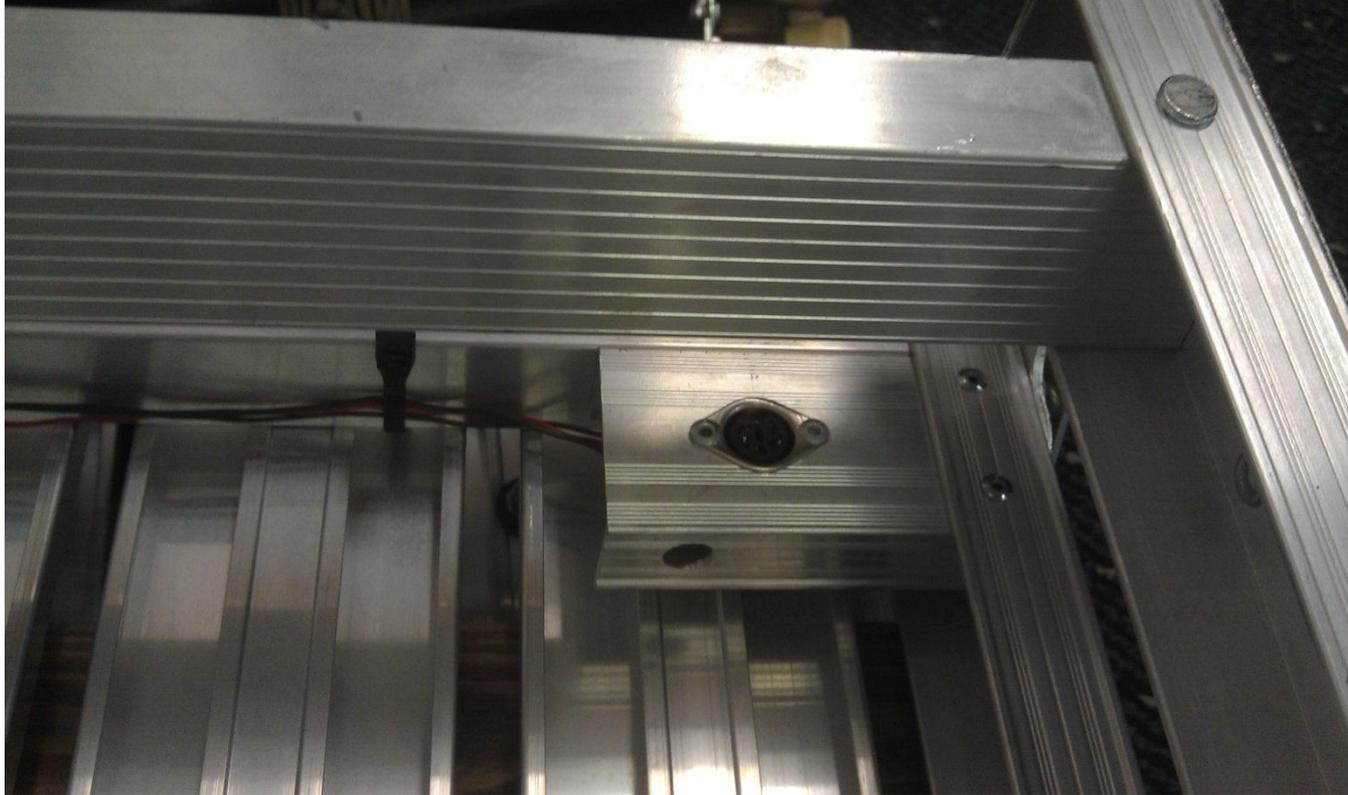
Alternative connector mounting. The extra switch legs can be used to mount the connector to the underside of the bench. This keeps the connector out of the way but makes it a little more difficult to set up and tear down
