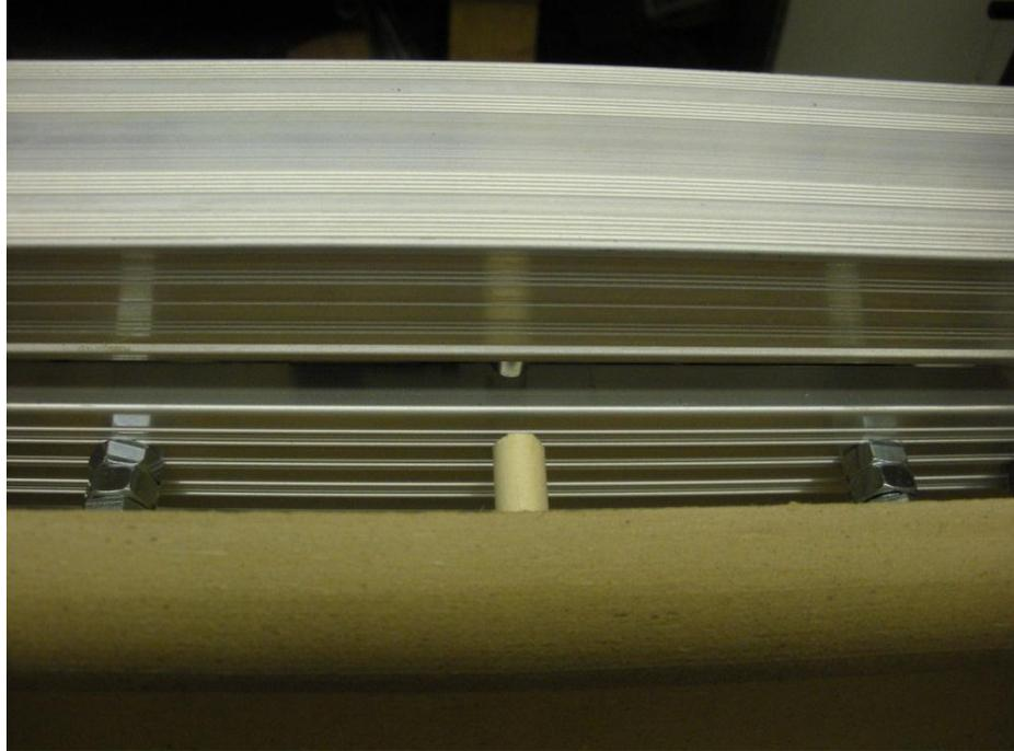
Cut dowel to size and dry fit in mounting hole. Make sure dowel does not over travel switch when seat is fully traveled down. Adjust by sanding or filing and then glue in place.
