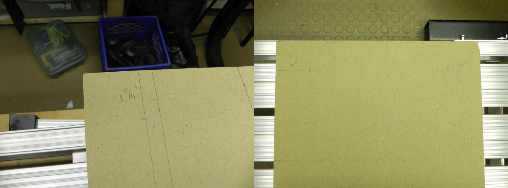
Mark holes for hold down/spring bolts at rear edge of seat. These holes are app  $1 \frac{3}{4}$ " from edge on the 4" line marked earlier. These holes will be app 2" from sides of seat when viewed from the top
