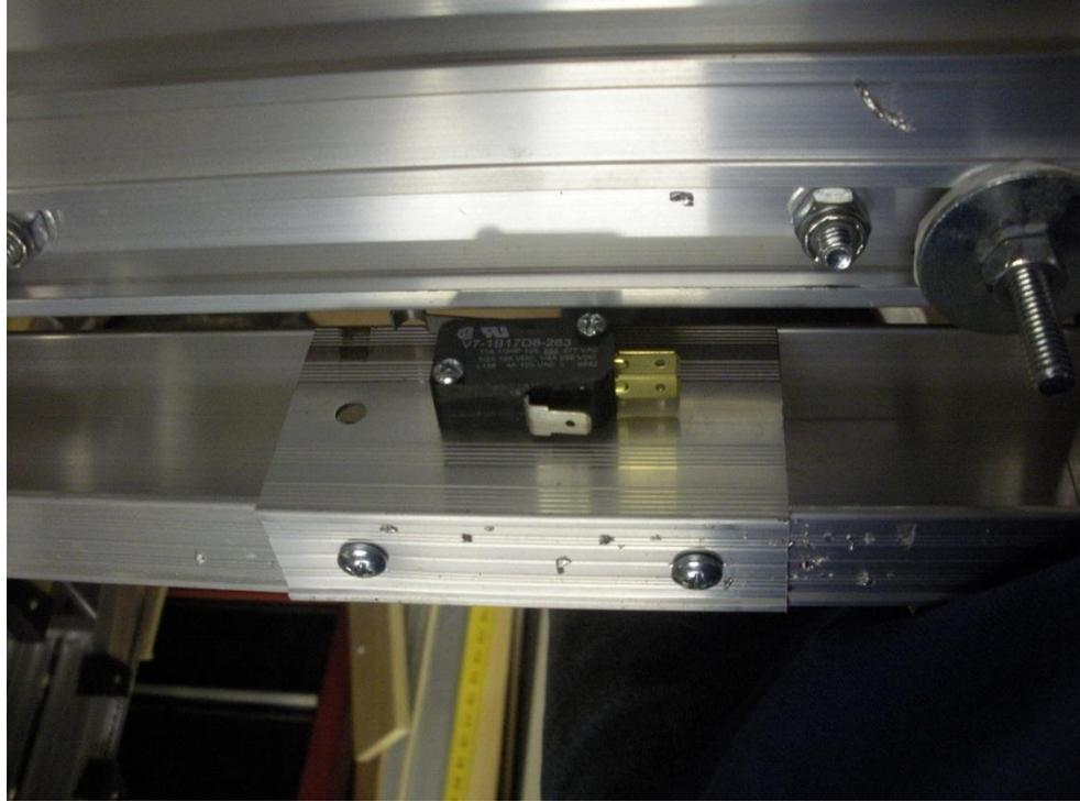
Tighten hold down/spring bolt bring seat down until dowel is just in contact with switch. Make sure switch is not overtraveled when seat is fully down.
