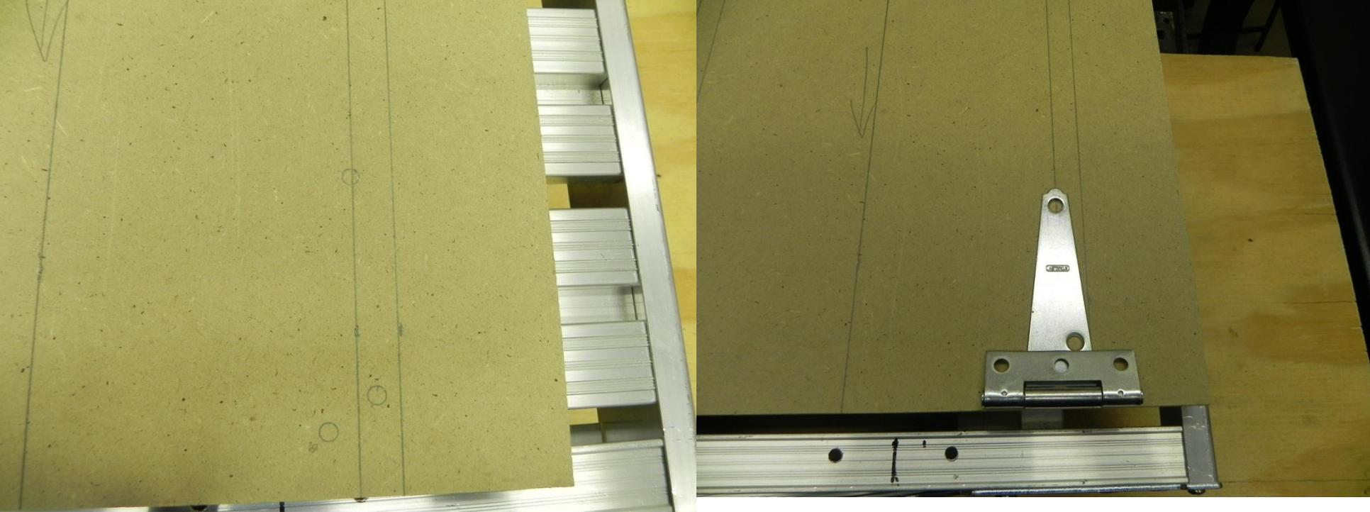
Place hinges on the backside of the seat and mark mounting locations. Drill holes and attach hinges to seats.
