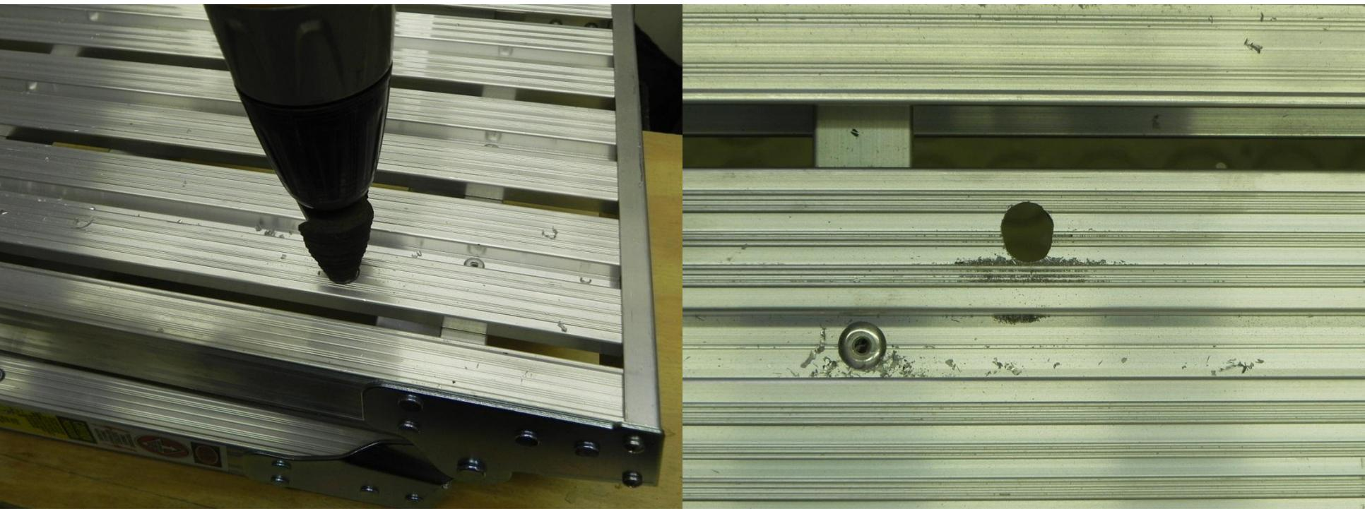
Drill holes for hold down bolts to pass through. These holes will need to be oversized and oval to allow bolt to pass through. I used a file to lengthen them fore/aft until the bolt would swing through and have clearance
