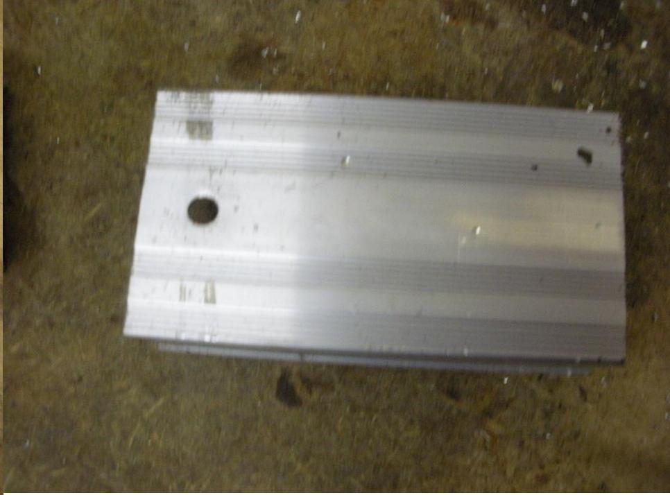
Use excess leg removed earlier for switch mounting. Place switch on leg and mark hole mounting locations. Drill holes and attach switch – rivet or small bolt/nut.
