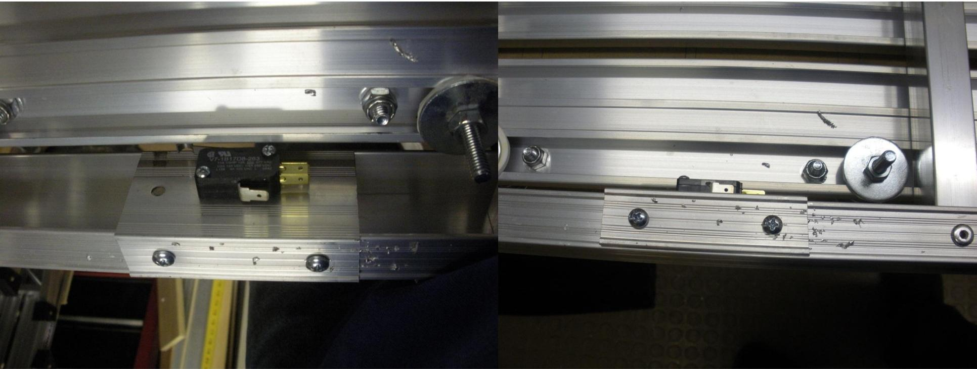
Attach leg piece with switch to bench making sure to align switch contact with hole in seat. I used self drilling screws to make repair easier later
