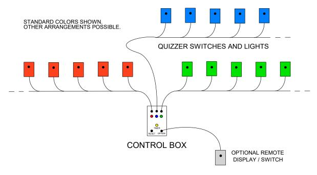
This quiz system will indicate the first quizzer to respond by turning on their light, locking everybody else out, and sounding a tone. Their response can also start a built-in timer, that can be used for time to complete an answer, time to speak the first few words, or both.
